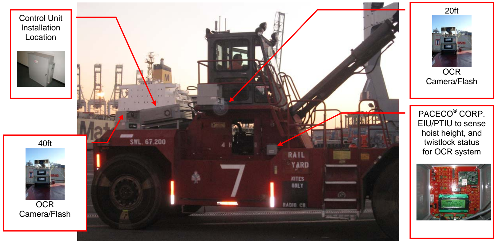
Figure 1 – Front End Loader With OCR Sensing Solution Installation Locations
