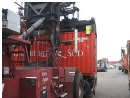
Fig 2 – Container Being placed onto an awaiting Chassis
